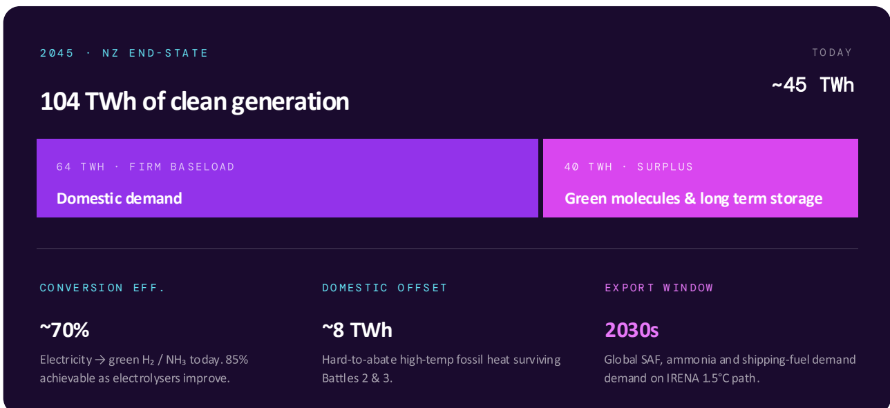
Figure 5.4.2 — NZ Prosperity scenario: 104 TWh by 2045, with 40 TWh of near-zero marginal-cost surplus producing clean molecules.
